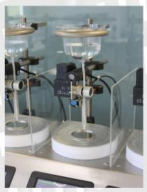
Contactless water level measurement Compact system: 4, 6 or 8 ways Homogeneous dry deposition
